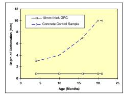
Comparative Depth of Carbonation in Accelerated Testing
